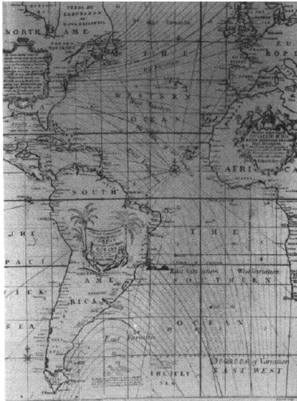
Isolines showing the deviations of compass
